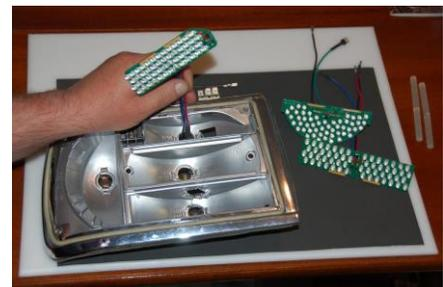
The circuit boards are secured to the fixture using RTV silicone or a Hot Glue Gun which is preferred because of its fast setting time. Just a 'tack' on all 4 corners is all that is needed, of course a glue or epoxy may also be used but this makes removing the array in the future more difficult.
