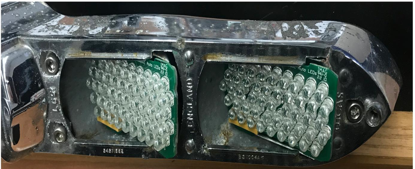
*How to fit the boards in the tail lamp housing
